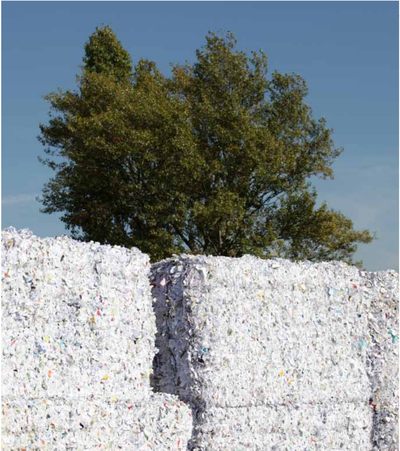
Once compacted, the different paper grades come out in bales measuring approximately one cubic meter, each weighing almost 900 kg.
