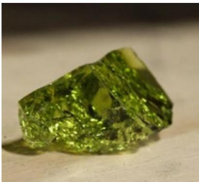
GeoMelt® creates ultra-stable glass that is typically 10 times stronger than concrete, and more durable than granite or marble. Its leach-resistance is among the highest of all materials in the world. Thus, a radionuclide trapped in the glass matrix will no longer be released into the environment, even after years of runoff.
